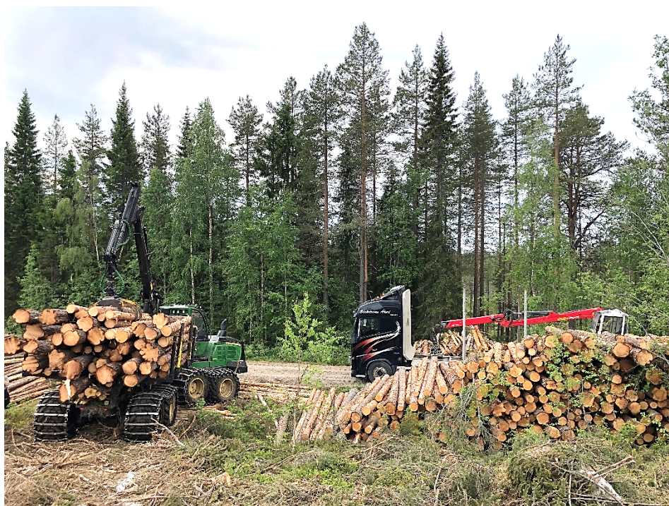
Fig. 27. The forwarder brings timber to the forest road. The timber is loaded onto a truck which takes it to the industry. Kamsjö, Västerbotten. Photo: Erik Normark.
