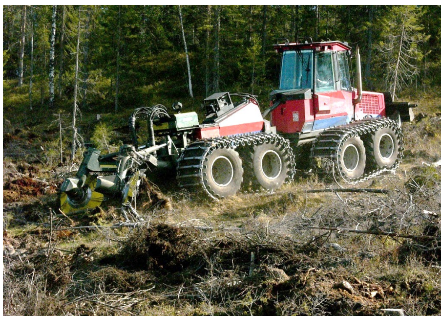
Fig. 20. Scarification of a clearcut. Gideå, Västernorrland. Photo: Erik Normark.
