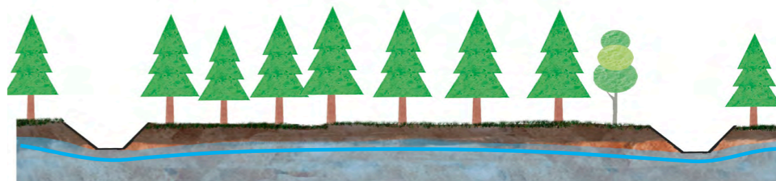
2. The condition after ditches are dug. The groundwater level has been lowered. Drainage effect decreases with distance from ditches.
