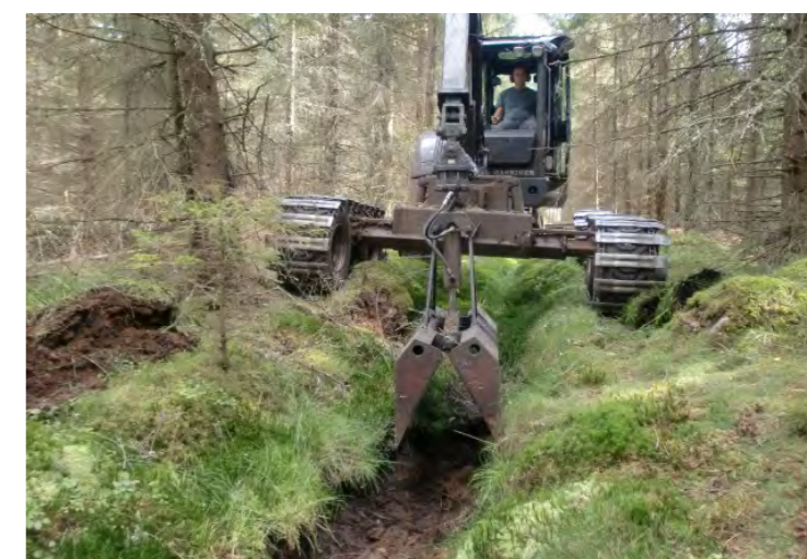
In the photo to the left, a profile bucket is used to remove accumulated debris in a ditch. In the photo to the right, a specialized machine with a cutting bucket is shown. Photo: Anja Lomander
